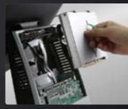
CPU module can be extracted for efficient upgrades and maintenance
